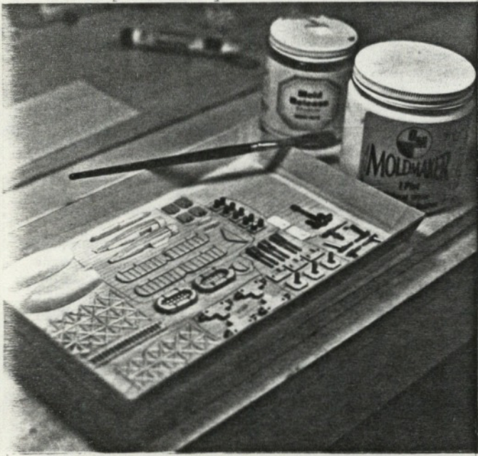
Original form. Parts include anchor, guns, bits, doors, boats, rafts and yes.. an airplane that molded very well.
