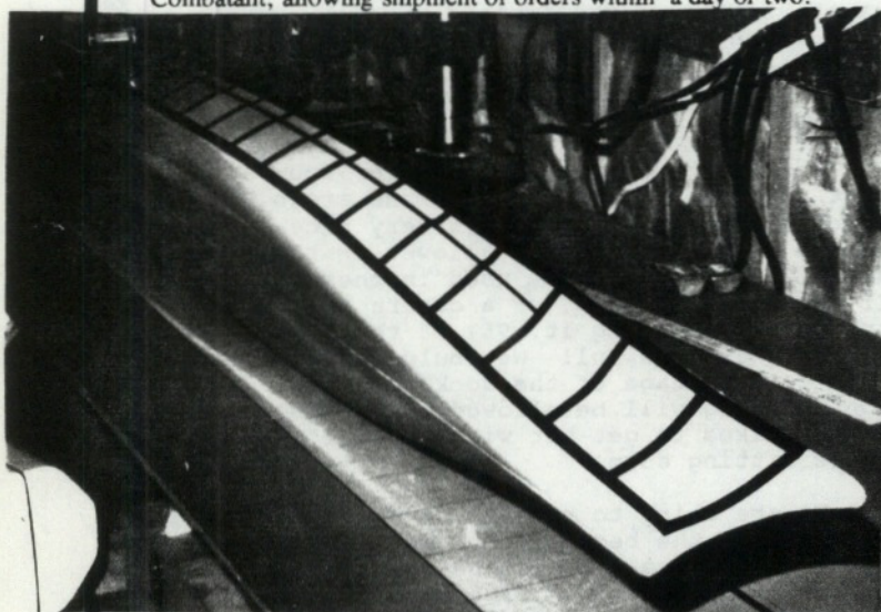
PHOTO 1 DKM BISMARCK hull being prepared for cutting. 3/8 inch electrical tape shows rib location, top, and bottom of penetrable area. 1/8 inch tape shows stringer at top of armor belt.
