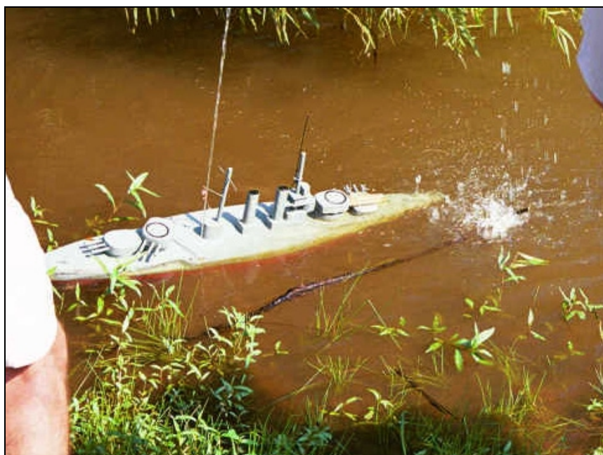
This Viribus Unitas displays the low freeboard in the forecastle that was a problem in her prototype.
