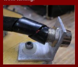
I also added a blinking green light for the bow and a blinking red light for the stern so I would know my orientation in the water. These were not permanent but were taped onto the ship when I needed them. I also added Dean's Mini Connector to the bow and stern lights. I wasn't happy with the
