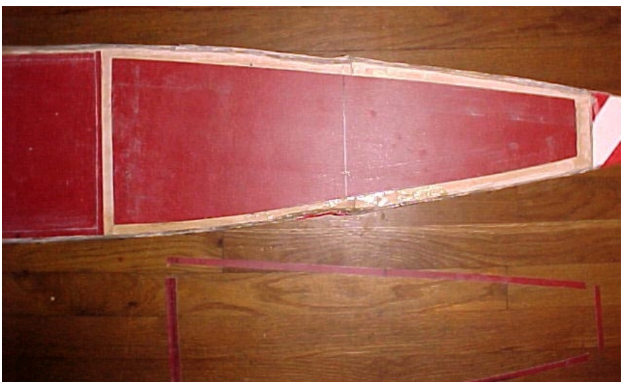
Step 4: Mark where the removable deck will be.
