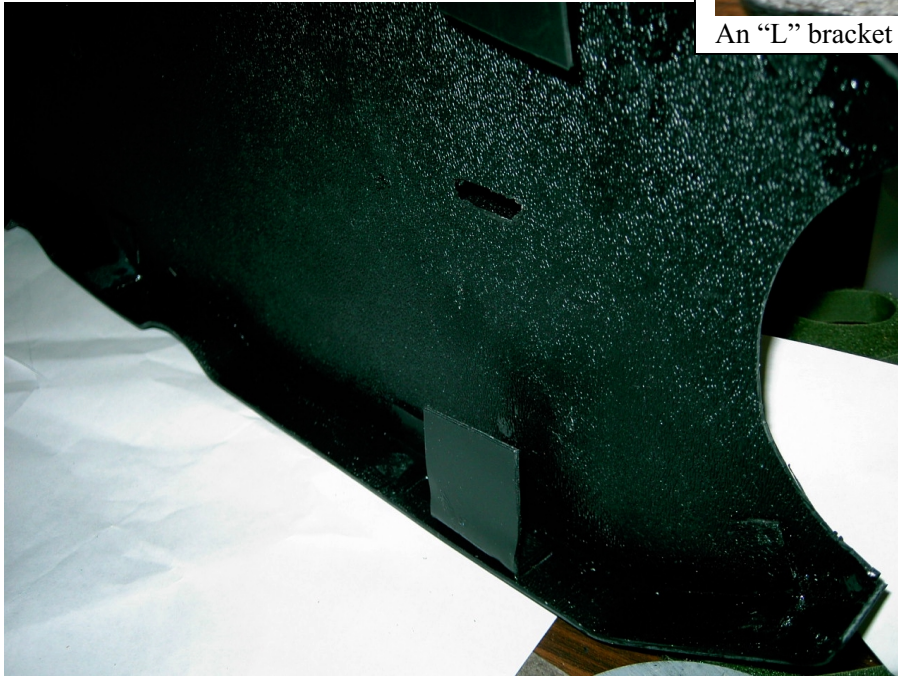
The bottom of the first deck. You can see the "L" bracket I will use to bolt this to the deck. You can also see some "L" brackets glued into place holding the vertical section to the deck.
