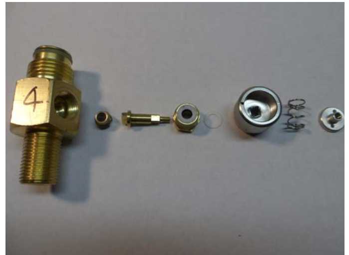
Upper L to R: Valve Body, Seal Screw, Shaft, Shaft Retaining Nut, Washer, Knob, Spring, Knob Nut If you zoom in you can see the brass debris on the retaining nut Teflon ring. This debris is being ground into the Teflon by the rotating action of the shaft.
